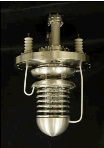
Fig. 1: A photograph of the field cage for the Argon gas-phase detector, which is mounted on the inside of the top flange of the argon chamber. The field cage encloses an active argon volume of 10 cm by 10.2 cm I.D. Proportional scintillation is generated in the 4 cm by 10.2 cm I.D. volume above the active volume. A collimated 100 \mu Ci ^{55} -Fe X-ray source is installed below the drift region volume, generating free electrons that drift through the applied electric field convert to proportional scintillation between two fine-mesh grids. This light is the detected by a Hamamatsu H6410 5.1-cm diameter photomultiplier tube.
