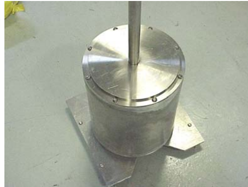
Figure 5 – Outer Container for the Neutron Irradiation Facility (NIF)
