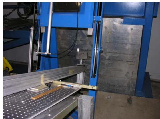
Figure 8 – Transmission measurement Experiment Set-Up for a Ni-Gd Plate
