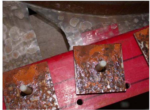
Figure 2 – Corrosive attack of 1018 carbon steel reference samples during atmospheric salt-fog test.
