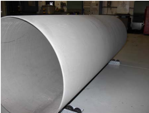
Figure 1 – Half-scale Type 316L stainless steel container coated with SAM2X5 Lot # 06-015, deposited HVOF with JK2000™ gun, photographed after atmospheric salt-fog test.
