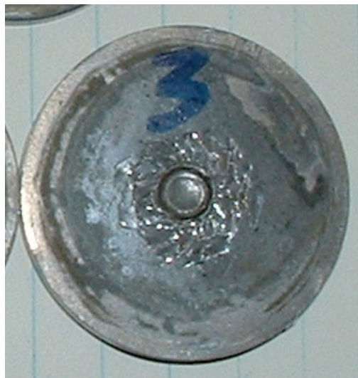
Figure 19. Photos of two representative lead witness plates from live M55 detonator testing at TACOM-ARDEC. The photo on the left a) is the dent left by an M55 stab detonator with an energetic nanolaminate stab mix/cyanuric triazide transfer charge and an output charge of EDF-2C. The one on the right b) is that left by an identical M55 stab detonator however with NOL-130 as the stab initiation mix.
