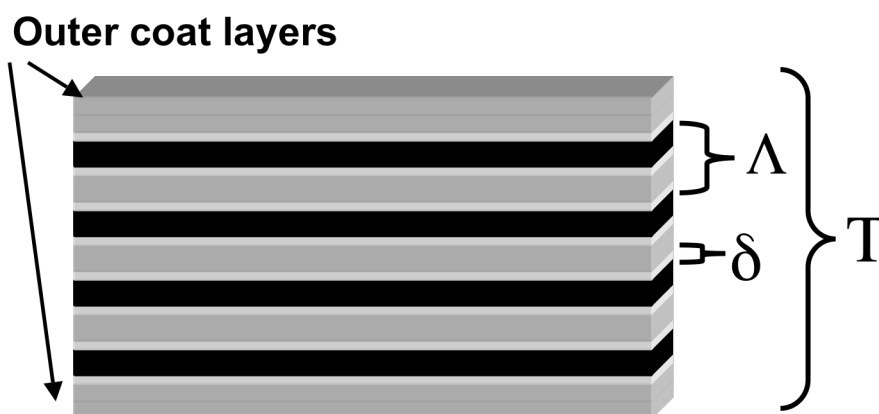
Scheme 1. Scheme showing the structural features of an energetic multilayer. The distance T_1 is the total thickness of the multilayer, \Lambda is the period or the repeating structural unit of the multilayer, and \delta is the prereaction zone
