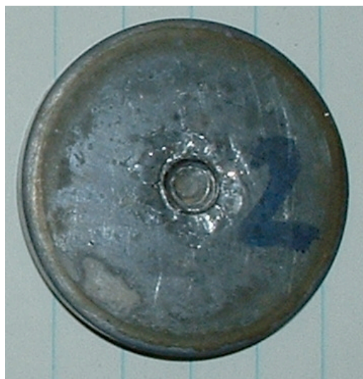
Figure 19. Photos of two representative lead witness plates from live M55 detonator testing at TACOM-ARDEC. The photo on the left a) is the dent left by an M55 stab detonator with an energetic nanolaminate stab mix/cyanuric triazide transfer charge and an output charge of EDF-2C. The one on the right b) is that left by an identical M55 stab detonator however with NOL-130 as the stab initiation mix.
