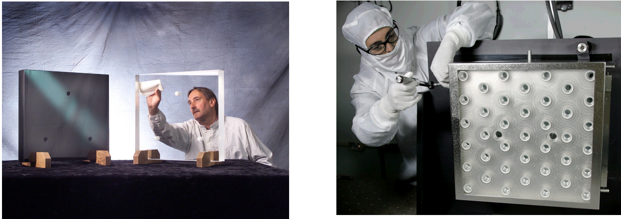
Fig. 4 Example of an unsolarized and solarized transport mirror (left image). NIF deformable mirror undergoing wavefront validation testing (right image).
