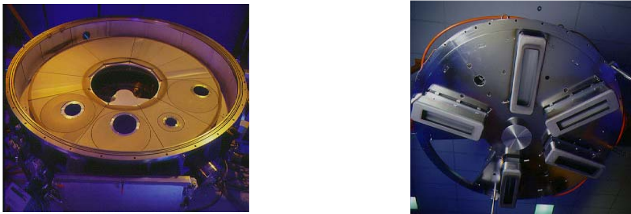
Figure 2: Left: View of substrate platter, with four silicon wafers of various sizes mounted on on-axis and off-axis positions. Right: Underneath view of chamber lid with five sputtering targets.
