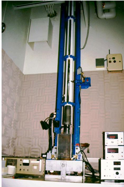
Figure 1. Drop hammer system at LLNL
