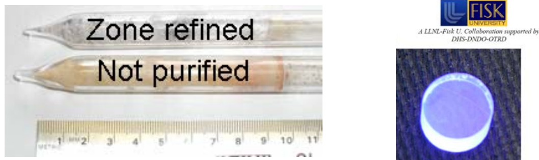
Fig. 1. (left) Photograph of two Barium Iodide boules, showing the removal of a brownish coloration upon zone refining. (right) A \text{BaI}_2(\text{Eu}) crystal grown from zone-refined materials under room lights and under UV illumination.
