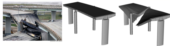
Figure 16. PARADYN FAILURE ANALYSIS COMPARED WITH PHOTO (PHOTO BY LACY ATKINS/SF CHRONICLE).
