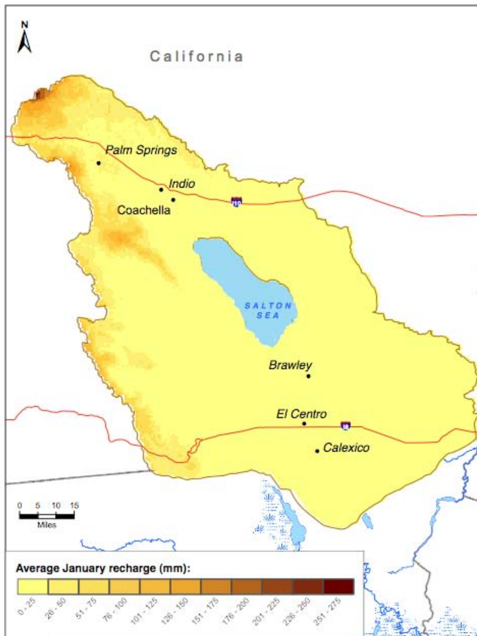
Figure A.1: Total precipitation excess in the Salton Sea watershed for the month of January, \Delta W_{PE}^{January} [mm], as calculated from (A.7) using the climatic normal data from 1991-2000 for the month of January. Recall, these do not reflect the effects of runoff (R) or other losses.
