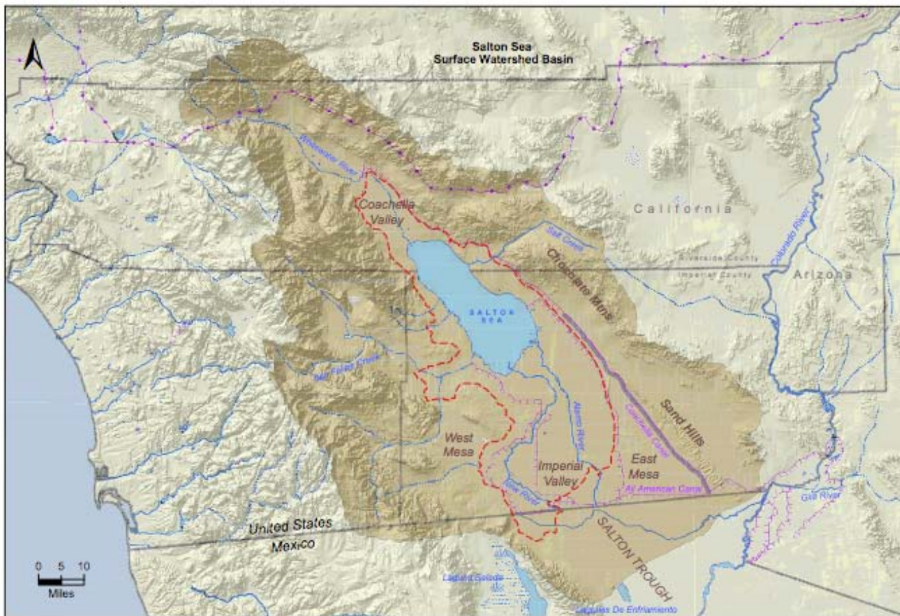
Figure 2.1: Map of the greater Salton Sea area in Southern California and Baja California Norte, similar to Figure 1.1, but showing the sea level elevation contour within the Salton Trough. The shaded area corresponds to the regional watershed basin, 8360 \text{ mi}^2 ( 21,700 \text{ km}^2 ) in area. Imported water aqueducts are shown in purple. The thick gray line indicates the lined portion of the Coachella Canal.
