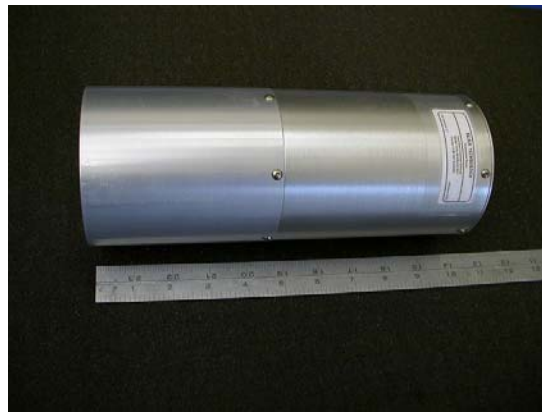
Figure 1. Photograph of a 4" diameter x 3" Eljen EJ-301 xylene based liquid scintillator detector with integration PMT.
