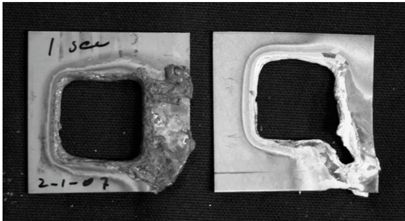
Figure 6. Thin titanium sheets (2" square) demonstrates combustion after laser turn-off
