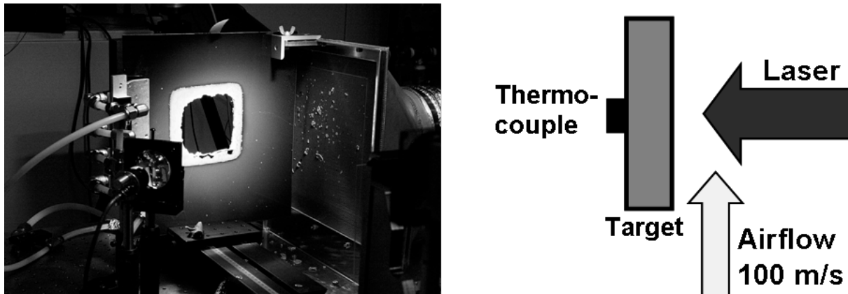
Figure 1. Experimental test setup and schematic representation
