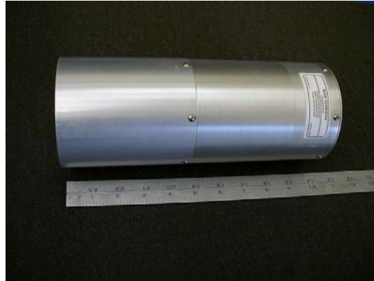
Figure 1 Photograph of a 4" diameter x 3" Eljen EJ-301 xylene based liquid scintillator detector with integration PMT.
