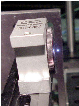
Figure 7: Focused 10W, 10kHz, 1mJ/pulse fiber laser beam. The bright spot behind the lens is a ball of plasma formed in the air through dielectric breakdown. This occurs at 10^{10} W/cm 2 .
