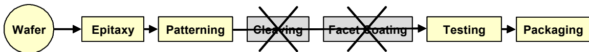
Fig. 3 Process flow for wafer-scale diodes eliminates cleaving and facet coating and facilitates early wafer-scale testing.
