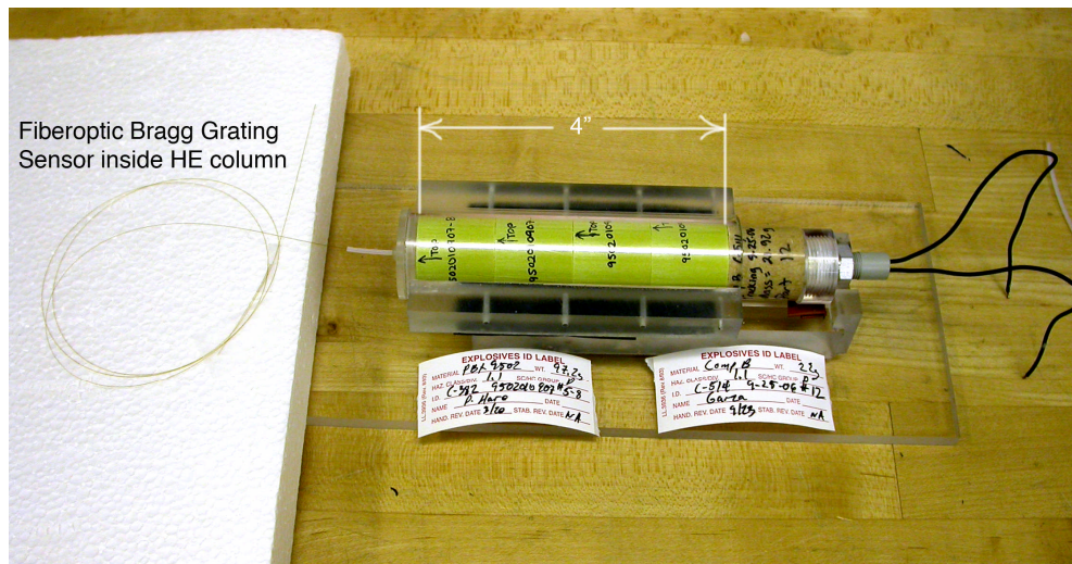
Figure 10. Experimental setup for PBX-9502 in-situ velocity test. Fiber-optic Bragg grating sensor is embedded in the high explosive.
