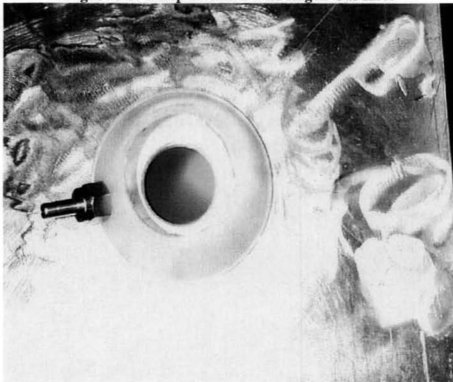
Figure 3-8. Sampler Collar with Argon Gas Inlet
