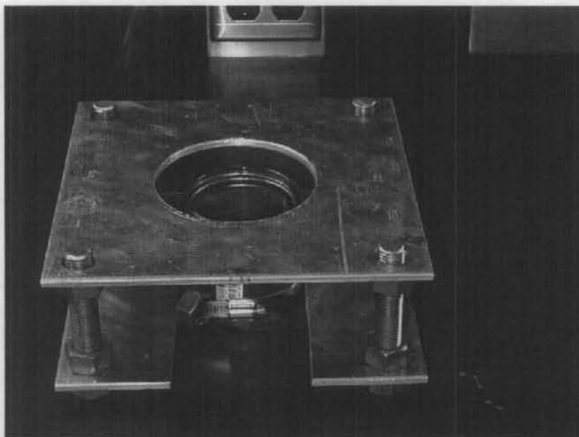
Figure 3-3. Middle Plate in Position
