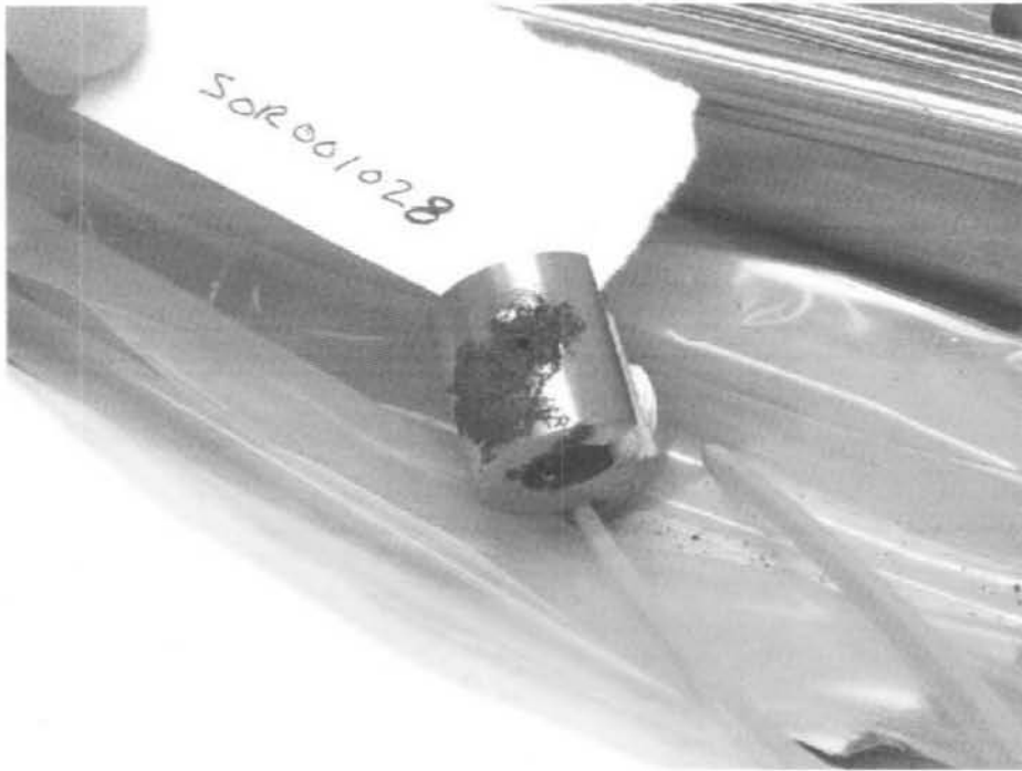
Figure 14. Macrophotograph of the Top of Vapor Space Nonstressed C-Ring S06R001028.
