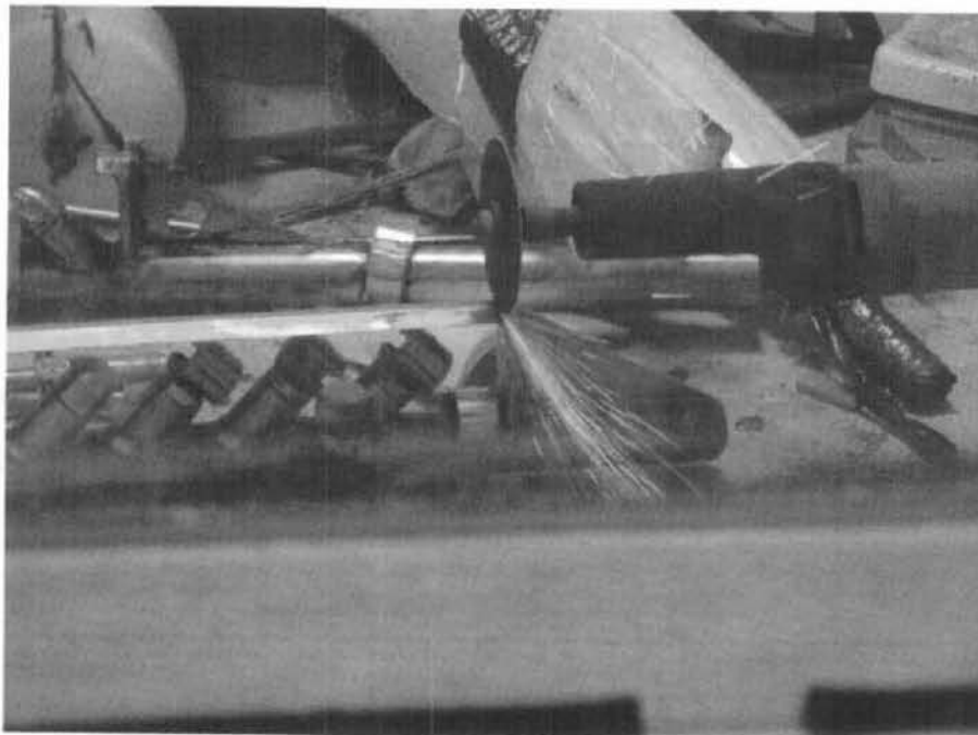
Figure 2. Removal of Cross Bar from Detector 4 in Hot Cell.
