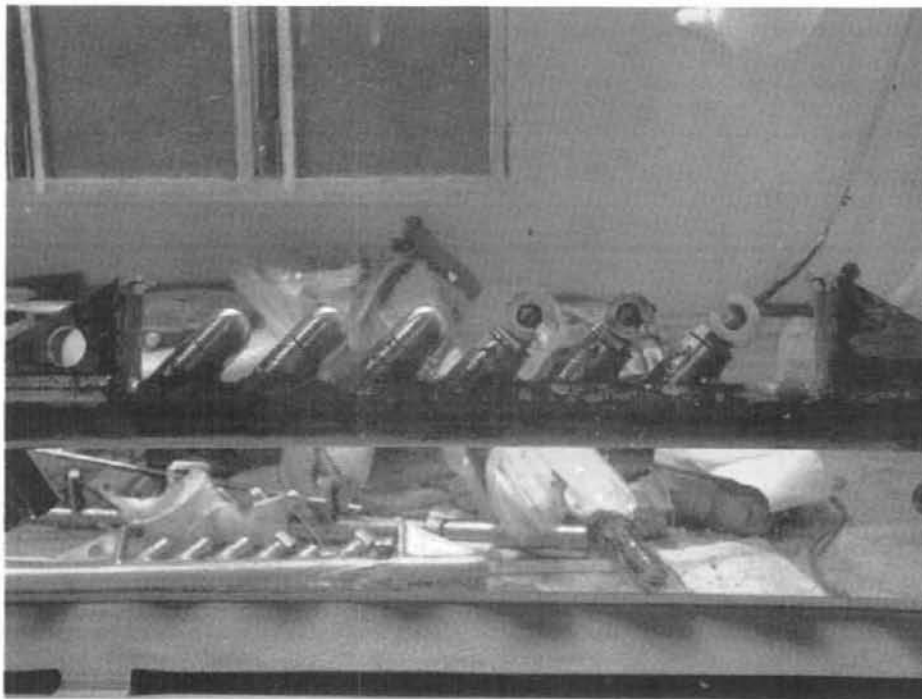
Figure 3. General View of Detector 2 During Disassembly in Hot Cell.
