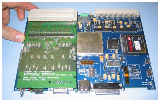
Figure 2 An FPGA motherboard is shown with one of its two analog converter mezzanine boards attached.
