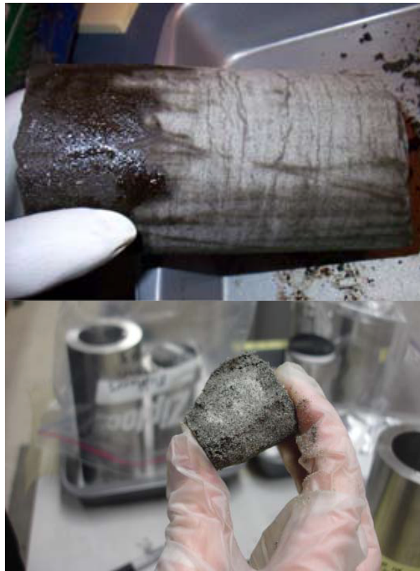
Figure 11 – Gas hydrate-bearing sand core and sample from the Mount Elbert deposit (Mount Elbert, 2007).
