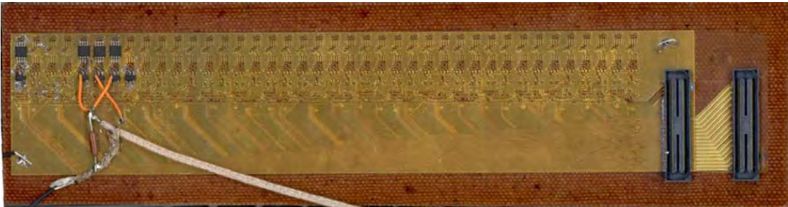
Figure 54: A prototype readout cable for the PIXEL.
