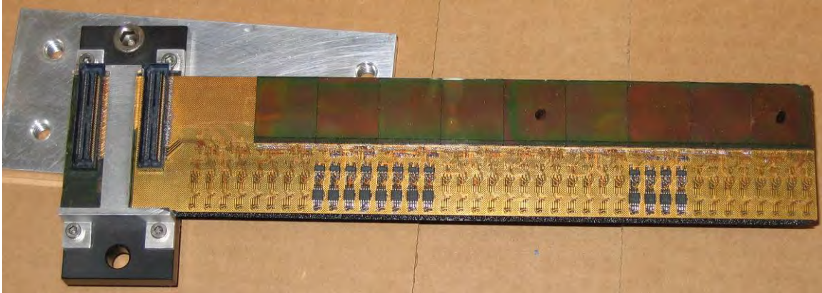
Figure 66: A prototype ladder showing low mass PCB, MIMOSA5 detectors and driver electronics bonded to a mechanical carbon fiber and reticulated vitreous carbon foam based carrier.
