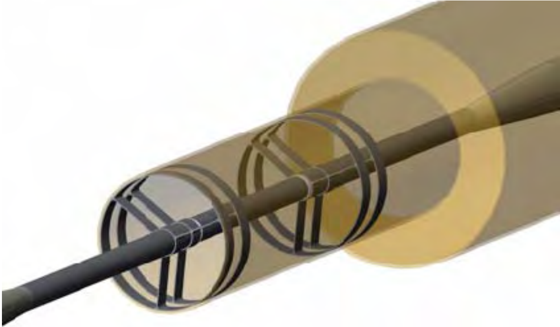
Figure 83: View of the beam pipe mid-section with central support.
