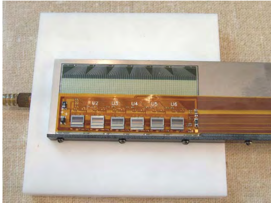
Figure 78: Prototype cable/hybrid, equipped with readout chips and mounted on a Type 1 PHOBOS silicon pad sensor.
