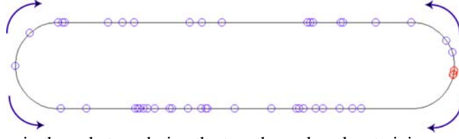
Fig. 4. Quench locations in the pole turn during the two thermal cycles: training quenches (blue markers), and plateau quenches (red markers). Both pole turns (inner and outer layer) are projected on the same plane. We refer to [16] for the detailed analysis of the quench locations.
