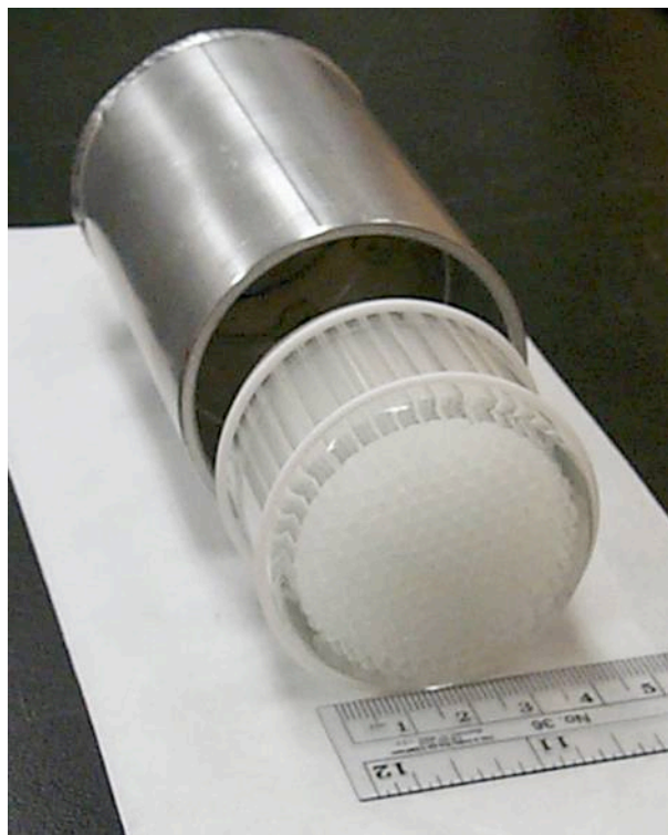
Figure 1 Prototype polymer coated glass (POG) passive sampler and aluminum housing
