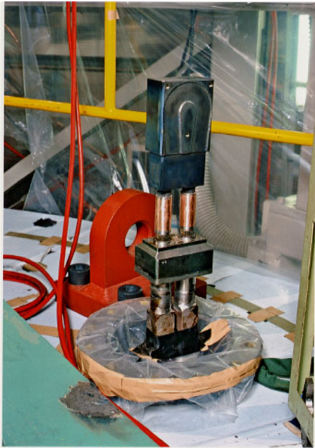
Fig.1. CSMC butt joint which joins two layers by a hairpin jumper, so two interfaces are in the joint. The joint interfaces are difficult to see after bonding. They are in the middle of the copper sleeves (Courtesy of Y. Takahashi).
