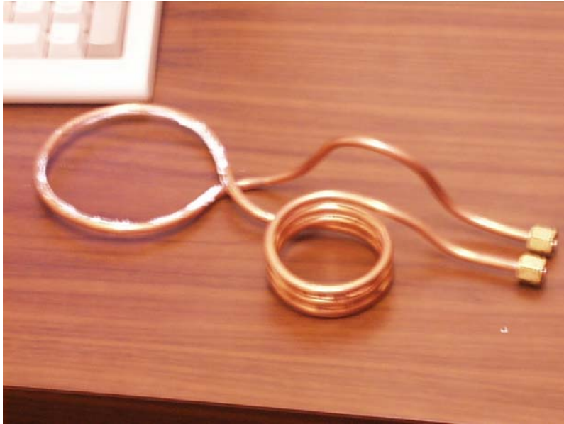
Fig. 10. An example of an induction coil with a parasitic inductance.
