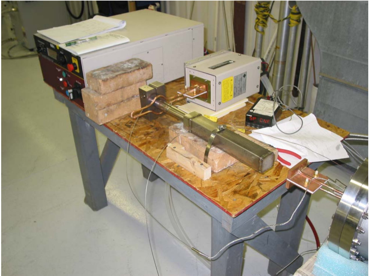
Fig. 9. A bench test with a clamp near induction coil to check heating efficiency.
