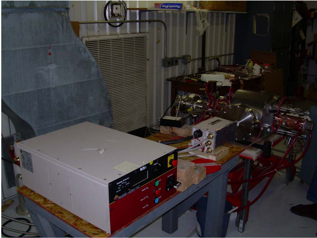
Fig. 4. The butt joint joining system shown from the side of the power supply and the remote station, connected to the induction heater coil.
