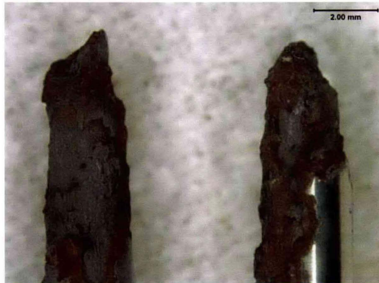
Figure 53. Stereo-Micrograph of the Test Sample from SSRT-75 Performed in AW-105-PSC 6X Simulant at 50°C, pH 13+, at a Potential of -50 mV vs. SCE.
