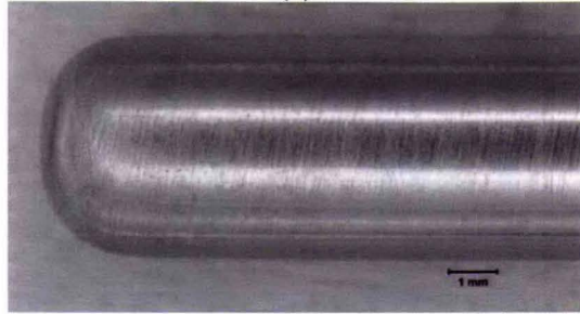
Figure B-27. The Appearance of the Sample after Exposed in AP105-PSC Purged with N 2 (Sample Partially Immersed, T=50°, EL1196-86).
