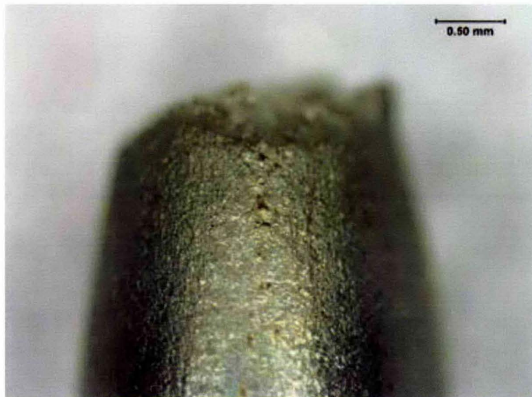
Figure 40. Stereo-Micrograph of the Test Sample from SSRT-57 Performed in SY-103-PIL Standard Simulant at 50°C, pH 14, at a Potential of 0 mV vs. SCE. The yellow dashed circles indicate axial microcracks observed on the shaft of the sample.
