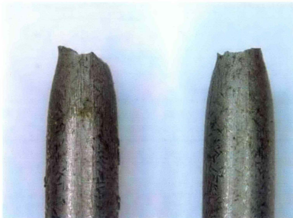
Figure C-8. A Stereo-Micrograph of the Sample from SSRT 49 Performed in AN107 Standard Simulant at 77°C, pH 13+ and at -790 mV vs. SCE.
