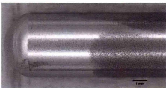
Figure B-31. The Appearance of the Sample after Exposed in AP105-PSC. The Head Space of the Cell Was Purged with N 2 (Sample Partially Immersed, T=50°, EL1196-96).
