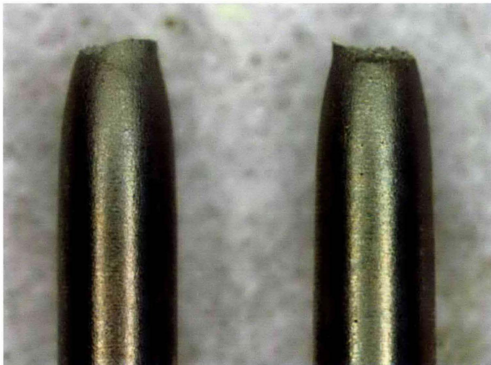
Figure C-32. A Stereo-Micrograph of the Sample from SSRT 57 Performed in SY103-PIL Standard Simulant at 50°C, pH 14 and at 0 mV vs. SCE.
