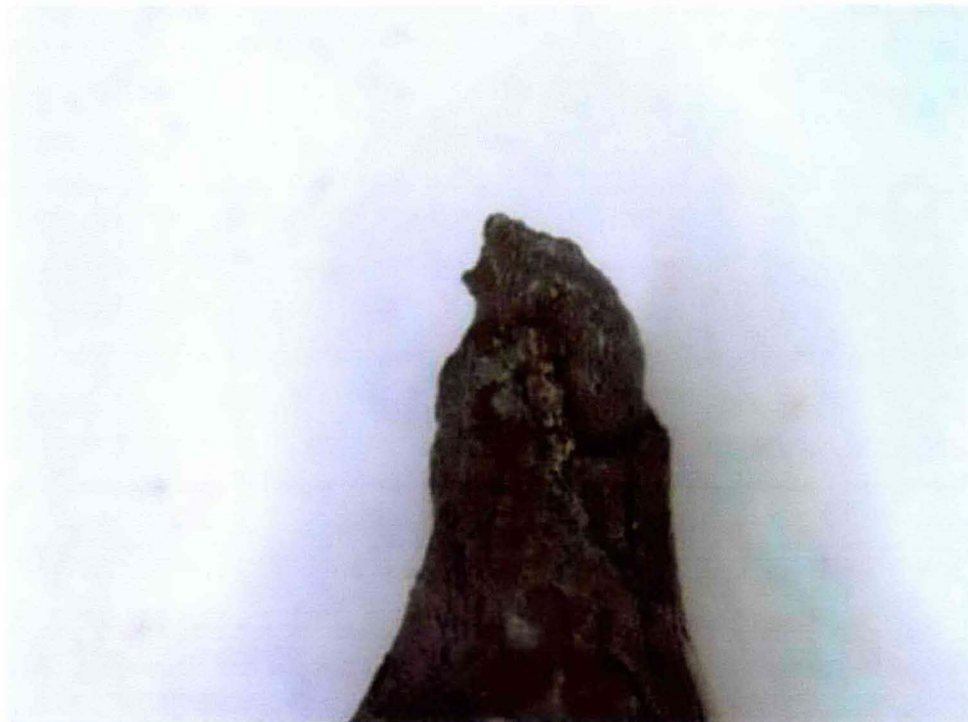
Figure C-11. A Stereo-Micrograph of the Sample from SSRT 50 Performed in AP105-PSC Standard Simulant at 50°C, pH 13+ and at 0 mV vs. SCE.
