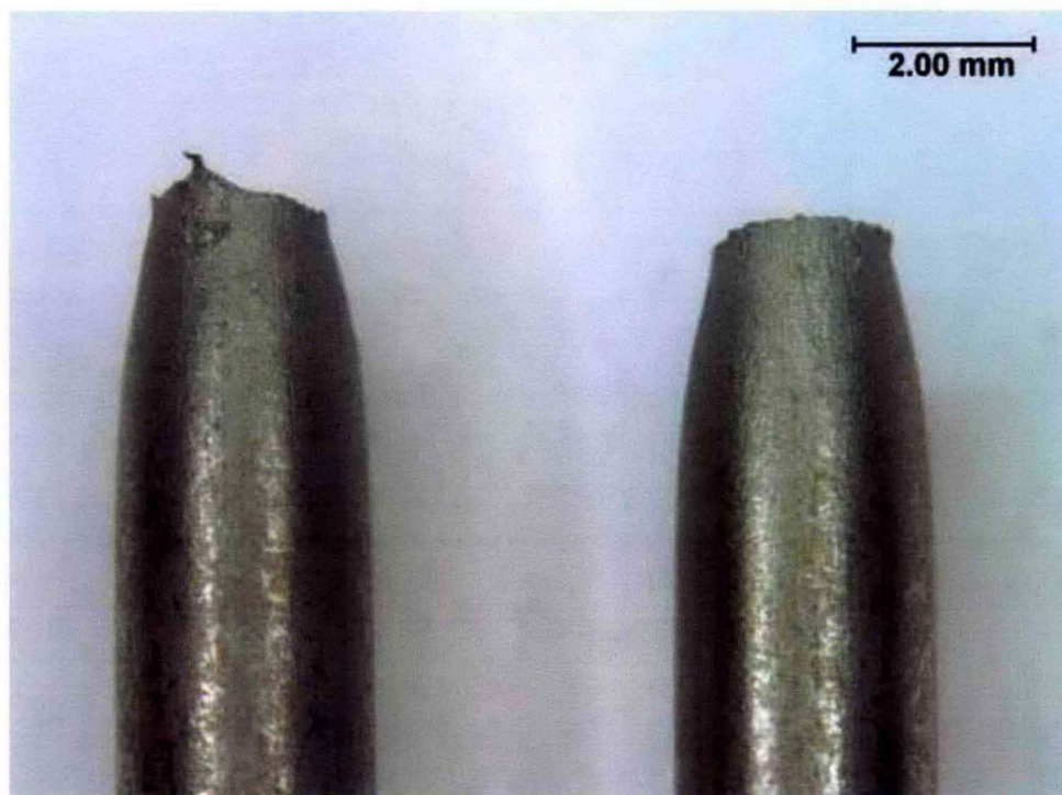
Figure C-2. A Stereo-Micrograph of the Sample from SSRT 47 Performed in AN107 Standard Simulant at 50°C, pH 11 and at -740 mV vs. SCE.
