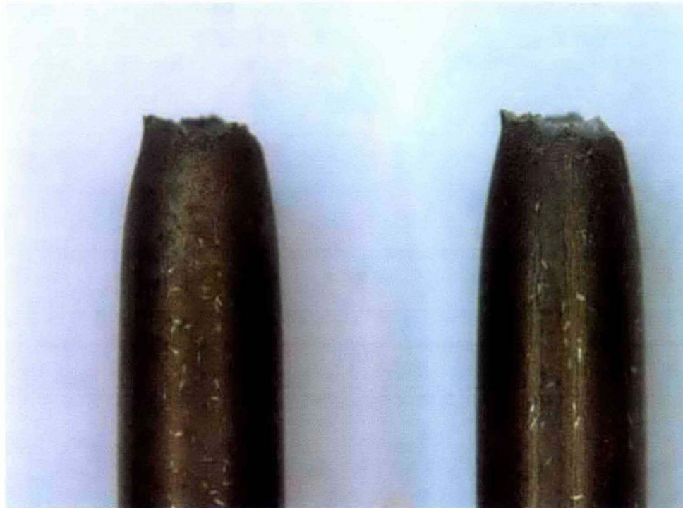
Figure C-5. A Stereo-Micrograph of the Sample from SSRT 48 Performed in AN107 Standard Simulant at 77°C, pH 11 and at -765 mV vs. SCE.
