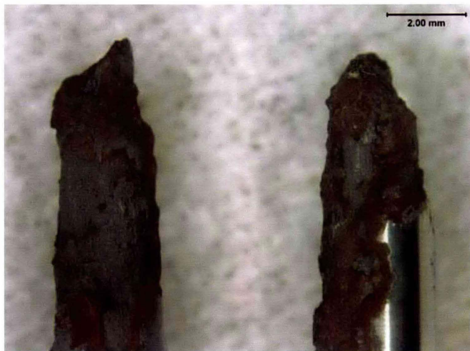
Figure C-79. A Stereo-Micrograph of the Sample from SSRT 75 Performed in AW105-PSC 6X Simulant at 50°C, pH 13+ and at -50 mV vs. SCE.
