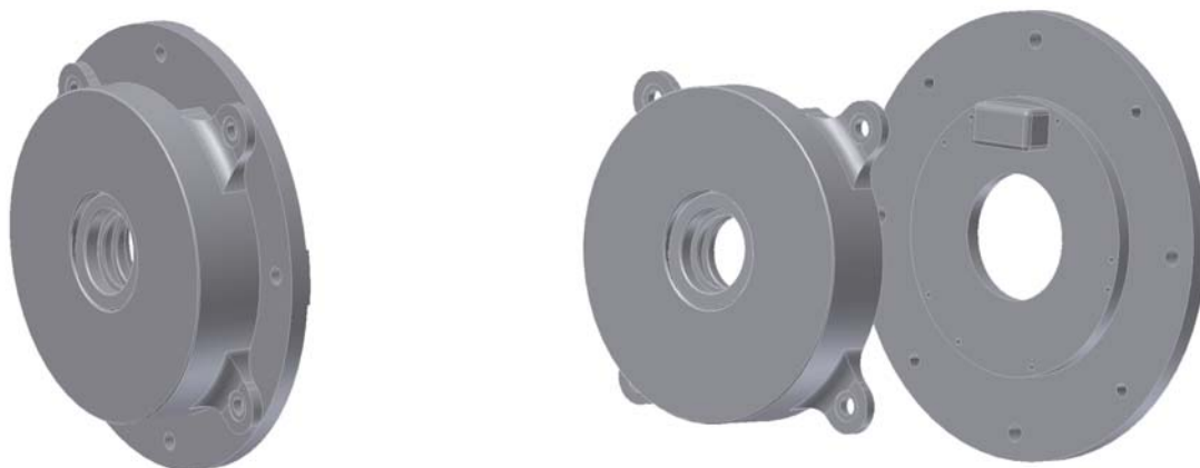
Figure 7-41 Entrance window and shutter (L: assembled, R: exploded showing shutter).
