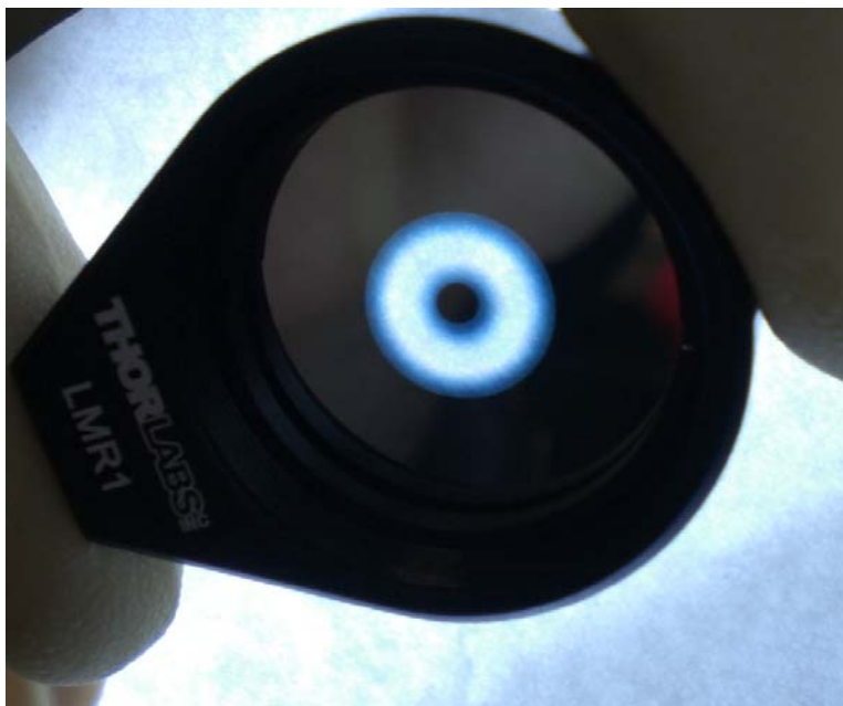
Figure 4-12 New Inconel Reynard apodizer at AMNH for AEOS pupil geometry. This will be used in an observing run immediately after GPI PDR to demonstrate on-sky performance of the APLC.
