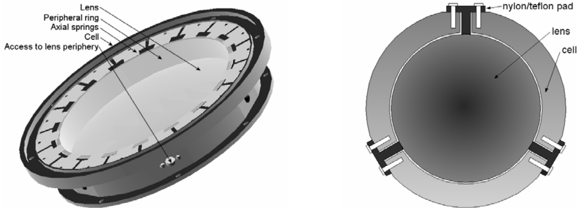
Figure 5.12 – Schematic view of the athermal lens mounting (left). The lens is held in place by an axial ring loaded by beryllium copper springs. One of the three accesses to the lens periphery, used for athermal centering, is shown in this schematic view. The view at right shows a cross-section of the mount. Nylon pads center the lens.
