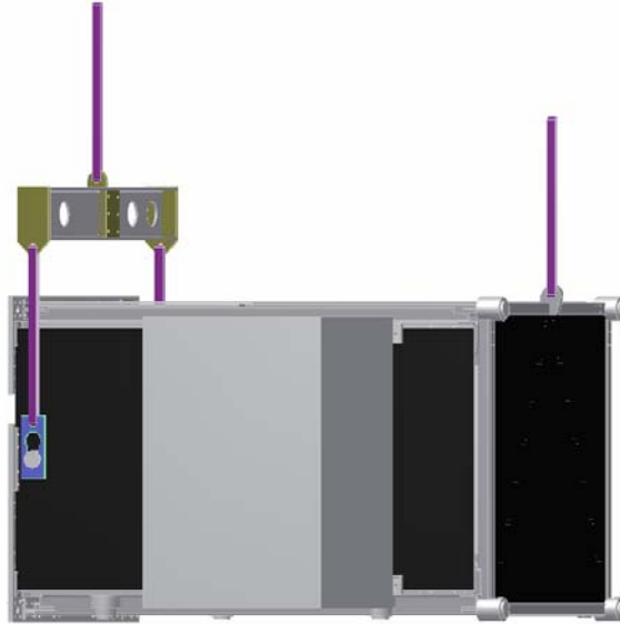
Figure 7-84 Lifting GPI for rotation to vertical.
