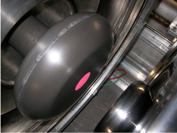
Figure 4: Photograph of the new cathode. The emitter surface is the red velvet at the center.
