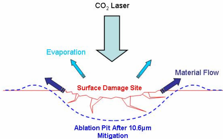
Figure 2: Drawing depicting the transformation of a damage site into a mitigation crater, indicating the removal of material via evaporation in the center (over an area roughly equal to the 1/e^2 of the laser spot), and a formation of a rim caused by mass movement along the surface.
