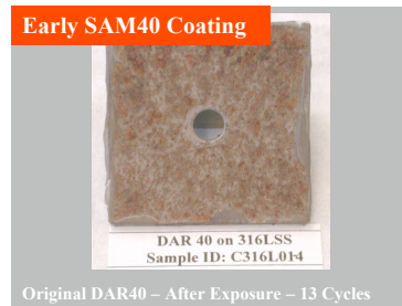
Original DAR40 – After Exposure – 13 Cycles
