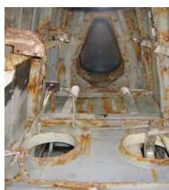
Internal Aft Sail Corrosion
