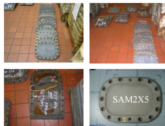
Sail Cover Plates Ready for Coating at Caterpillar
