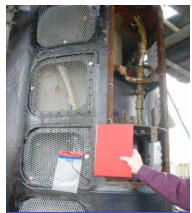
Exterior Forward Sail Cover Plates Removed
