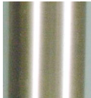
Tested for 243 hrs ASTM B117 Salt Fog
