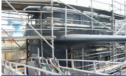
Sail of Ex-Portsmouth 688 Class Submarine with Black Epoxy Coating on Exterior Surface
