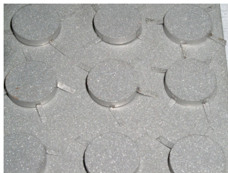
Example Corrosion Disks
