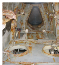
Internal Aft Sail Corrosion
