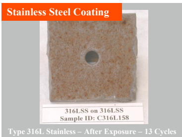
Type 316L Stainless – After Exposure – 13 Cycles
