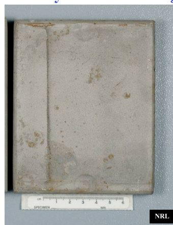
Early SAM40 Coating After Cavitation Testing
