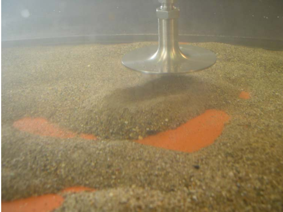
Figure 37 Close-Up Photograph of a Sand Mound Beneath the Solid Horn and Several Holes where Sand Removed
