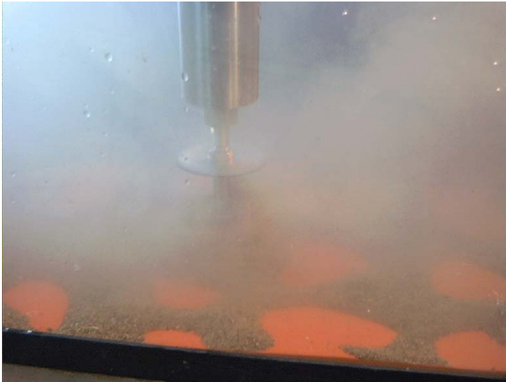
Figure 38 Photograph Illustrating Major Fine Sediment Suspension and a Complex Pattern of Several Holes Where Sand Removed
