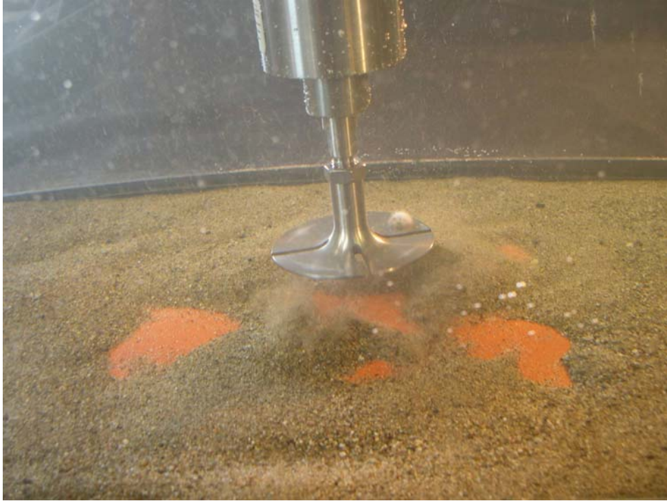
Figure 36 Photograph Showing Cluster of Cavitation Bubbles, Holes in the Sand Layer, and Minor Amount of Fine Sediment Suspension
