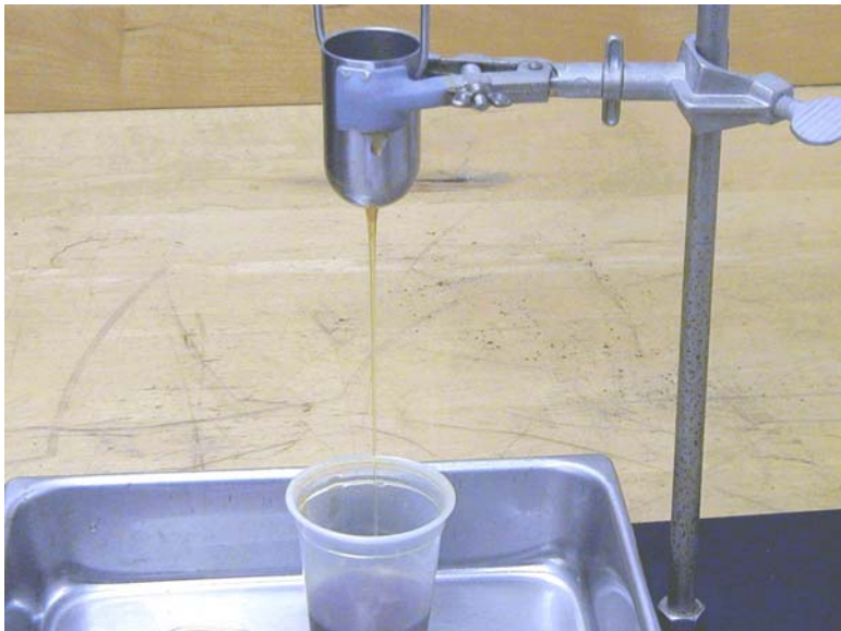
Figure 9 Photograph of Dip Cup for Measuring Viscosity
