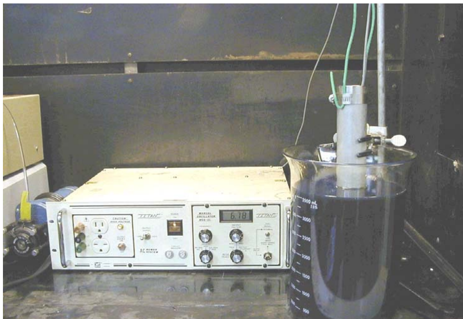
Figure 10 Experimental Setup During Acoustic Treatment of Oil
