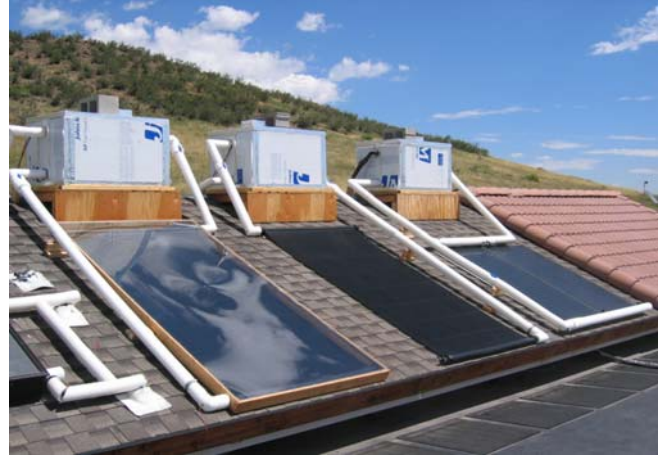
Figure 3. Three thermosiphon systems on test, with a glazed collector on left and two unglazed collectors to the right.
