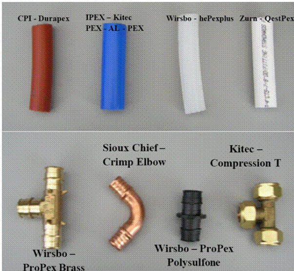
Fig. 6. Four types of PEX piping tested (top), along with some of the fittings tested (bottom).
