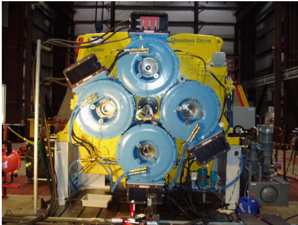
Figure 8. Clipper Wind Power's new 2.5-MW turbine incorporates an innovative distributed drivetrain.
