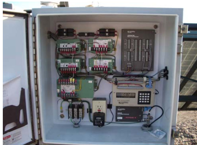
Fig. 2. Typical DAS using Campbell Scientific data logger.
