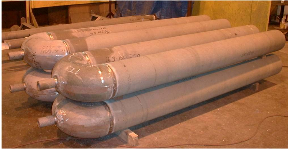
Fig. 4.32. Typical radiant-tube assembly fabricated using newly developed HP alloys.
