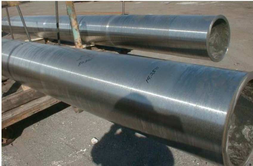
Fig. 4.33. Furnace roll cast at Duraloy Technologies from HK alloy developed in this project.
