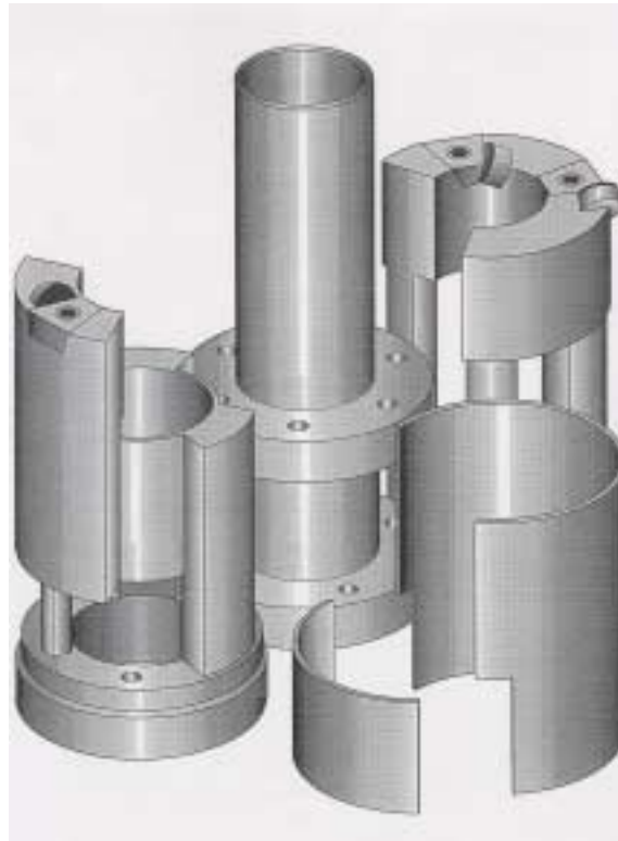
Figure 1. Breakdown view of the HRDF instrumented bit. Note that the test cutter is mounted in the section of the bit body shown at the left side of the image.
