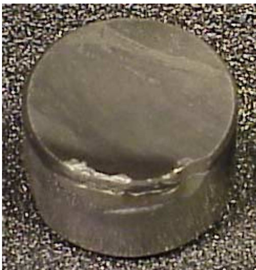
Figure 4a. Lightly-worn PDC at Stable Drilling Condition (96 ft of Sierra White Granite at 30 ft/hr, 2000 lb. WOB and 100 RPM).
