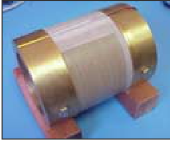
Figure 3. A piezoelectric transmitter for acoustic MWD.
