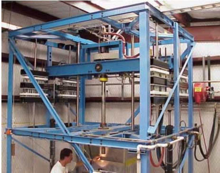
Figure 1. Sandia’s Hard-Rock Drilling Facility Modified to Include Axial Compliance.
