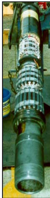
Figure 2. The Baker prototype with its cover removed showing batteries, microprocessor, coil and ceramic transducer.
