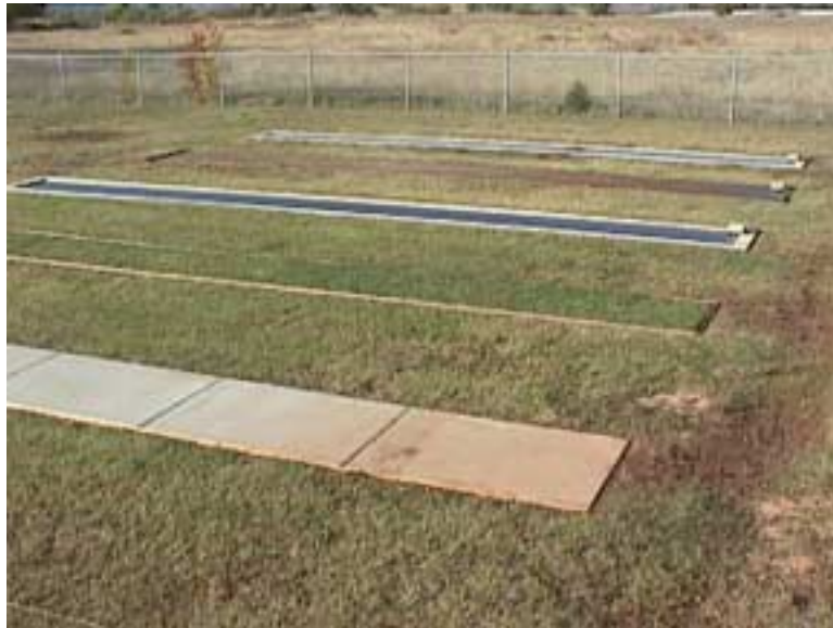
Figure 1. Five Shallow Heat Exchanger Systems.
