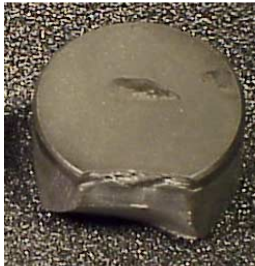
Figure 4b. Failed PDC cutter in chatter conditions (1 ft of Sierra White Granite at 10 ft/hr, 1500 lb. WOB and 140 RPM).
