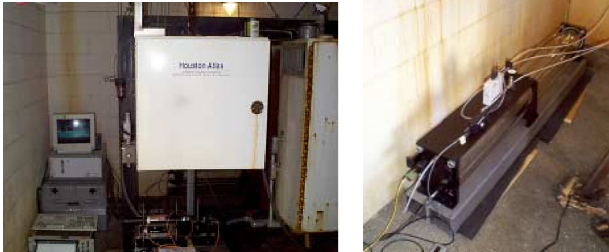
Figure 1. H 2 S Analyzer and Multi-Pass Sampling Cell Deployed Behind Houston Atlas Instrument at NCPA.
