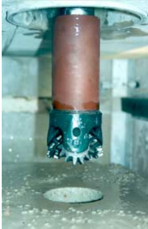
Figure 2. Rollercone bit used in HRDF to remove drillable straddle packer from cemented borehole.
