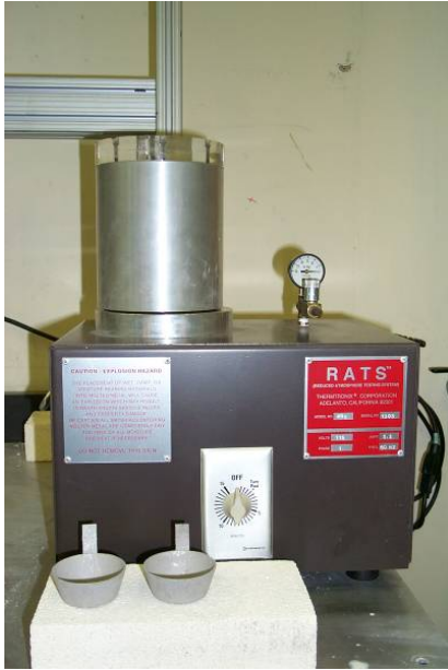
Fig. 4.3. Reduced pressure test (RPT) system used in this project for measuring the density of aluminum alloys processed by various degassing methods.
