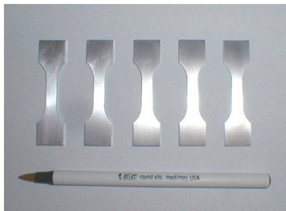
Fig. 4.16. Schematic ( top ) and picture ( bottom ) of the tensile and fatigue test specimens. Specimens were 2.54 mm thick. (All dimensions in mm.)
