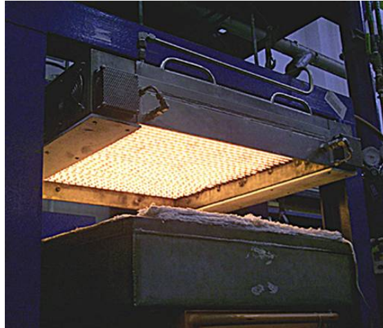
Fig. 4.4. ORNL's 88-kW batch-type drop-bottom IR furnace.
