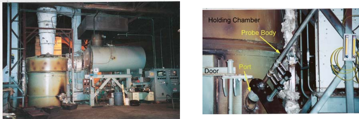
Figure 27 - Furnace Used for Mixing Tests
