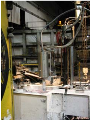
Figure 21 - LIBS Probe Installed at Commonwealth
