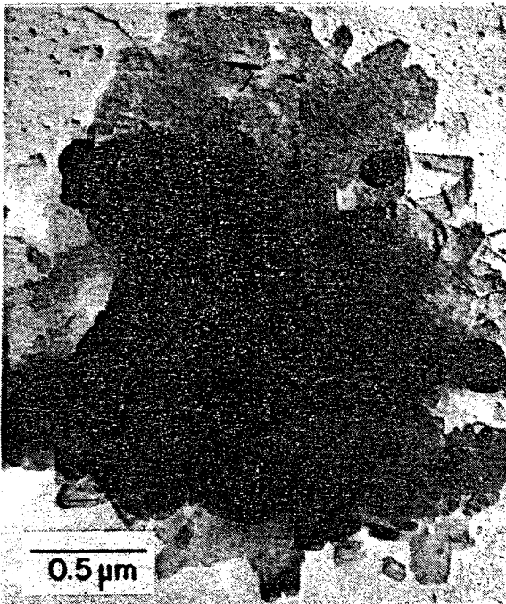
Figure 9. Platy smectite particles formed at 700°F in the attapulgite/water system.
