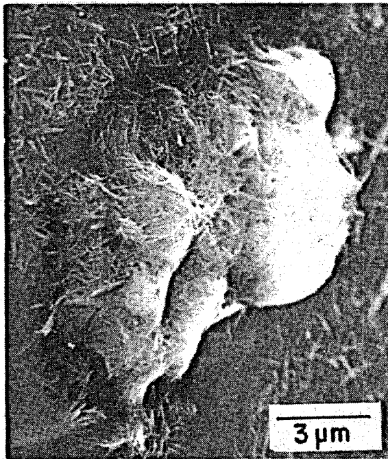
Figure 3a. SEM image of a thick and fluffy attapulgite aggregate
