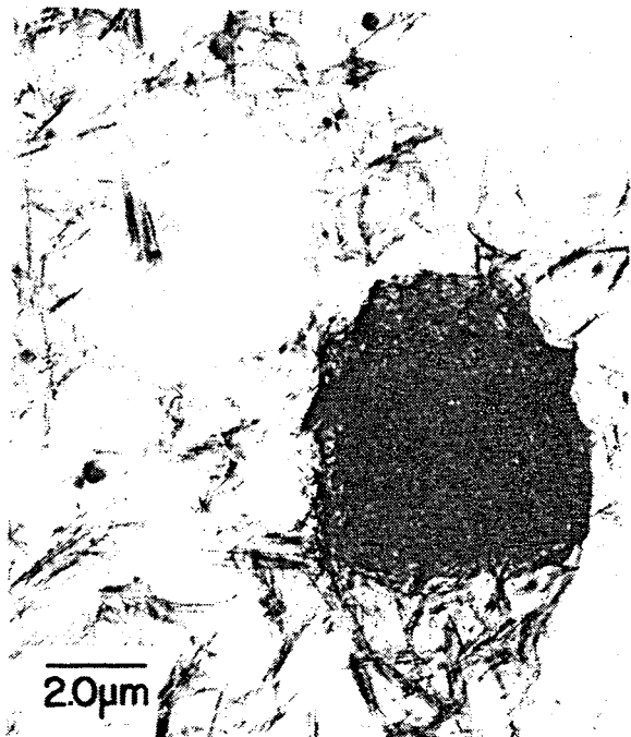
Figure 21. Aggregation of sepiolite fibers into spherical flocks during testing in FANN 50C viscometer.
