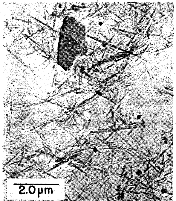
Figure 18. Dispersed sepiolite fibers in the slurry after being sheared at room temperature for 2 hours.
