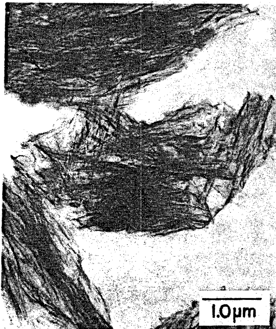
Figure 24. Aggregates of thin smectite films and original sepiolite fibers formed during testing at 500°F with FANN 50C viscometer.
