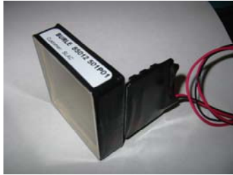
Fig. 1. Burle/Photonis “open area” 64-pixel MCP-PMT 85012-501 (S/N 11180401) with 10 \mu m hole diameter.
