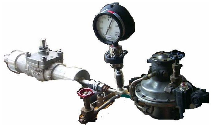
Figure 15: Hydrostatic Test of a Valve Identical to the Leaking Valve
