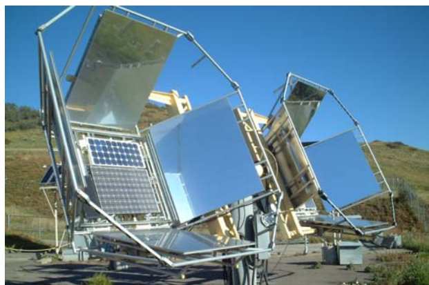
Fig. 1. The Outdoor Accelerated-weathering Test System at the NREL Outdoor Test Facility.
