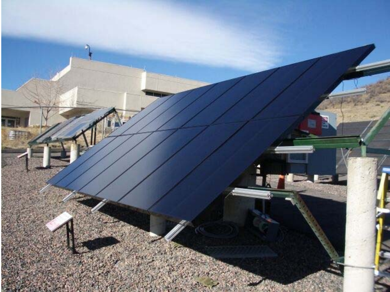
Figure 48. The fourth 1-kW array provided to the NREL Outdoor Test Facility. The array is comprised of 14 Eclipse 80-C modules.
