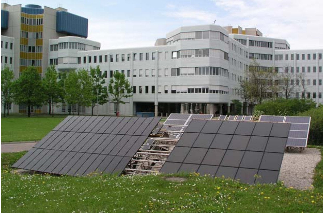
Figure 50. Photo of the outdoor test facility in Munich-Perlach. Several technologies are compared in a side-by-side arrangement.
