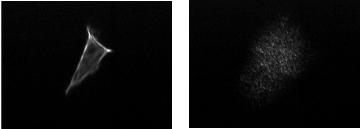
Figure 1. Example of real KDP back-reflection pattern (a) left image is without a phase plate (b) right image in the presence of a phase plate
