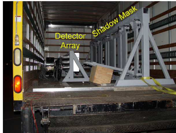
Fig. 1. The prototype imager is mounted in the rear of a rental truck. The image is formed from the shadow pattern cast on the 3 x 19 array of detector elements by the lead mask.
