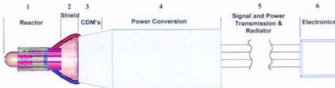
FIGURE 4.1: Electrical Cable Temperature Regions
