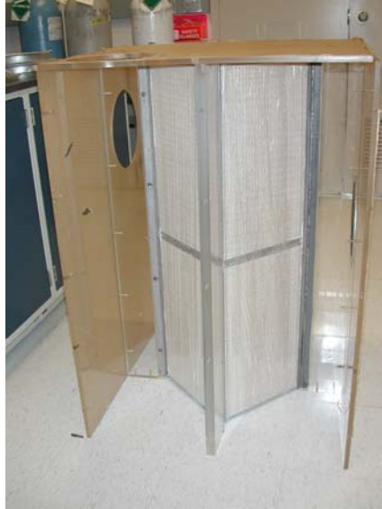
Figure 7.18. EERV core in custom Plexiglas® manifold. Protective paper has not yet been removed.
