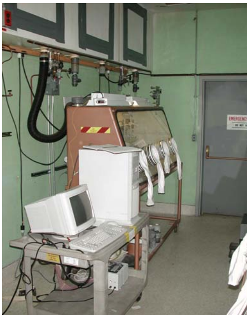
Fig. 2.3. Photograph of data acquisition system and glove box used for the experiments.
