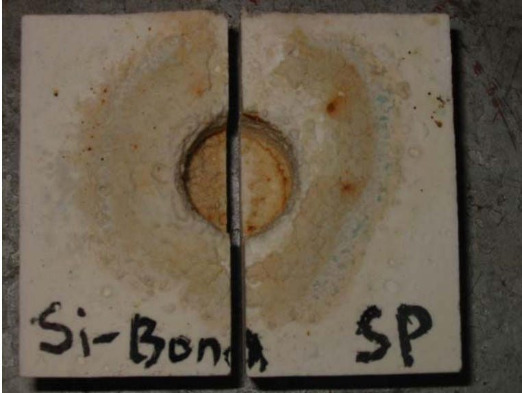
Figure 29 Top view of sample 26 after cup test.
