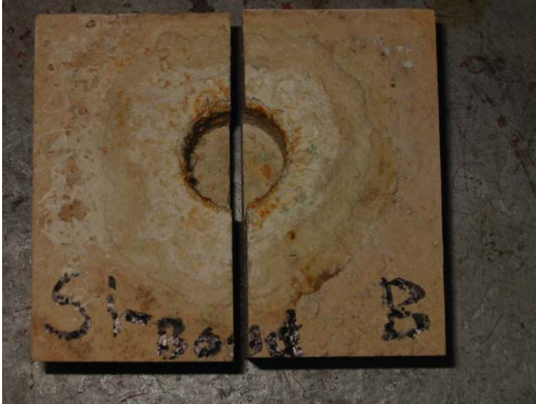
Figure 27 Top view of sample 25 after cup test.
