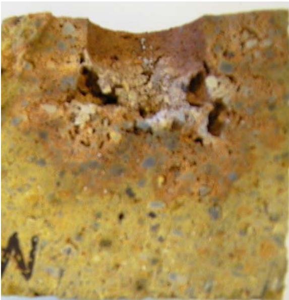
Figure 45 Bloating of magnesia castable mix.
