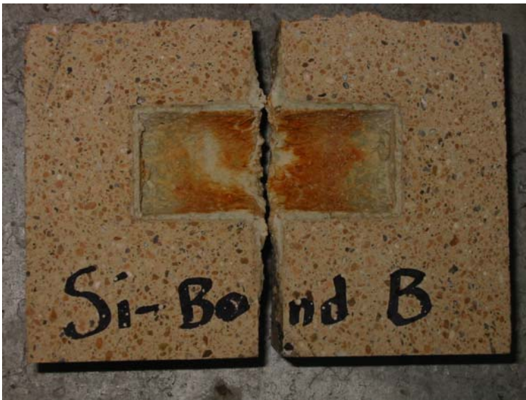
Figure 28 Cross-section of sample 25 after cup test.
