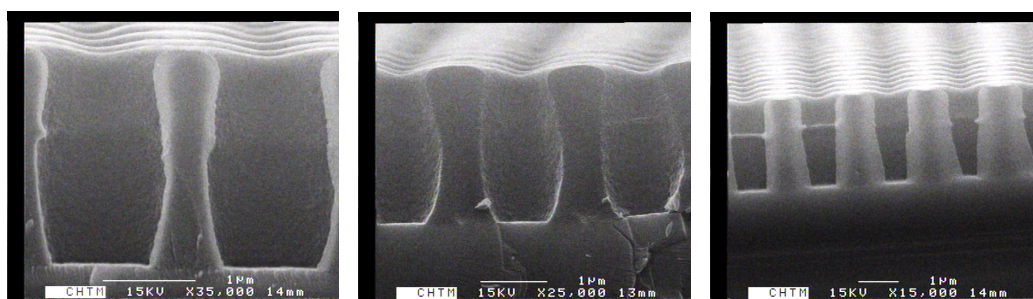
Figure 10. a) Top down SEM showing incomplete hole array, b) SEM showing of surface showing broken gold posts, and c) SEM of SU-8 film after removal indicating broken posts in film as well as void in the center of the hollow posts.
